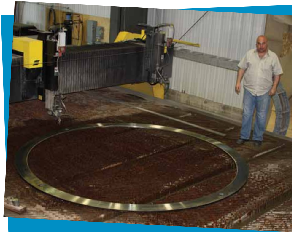
The KMT waterjet is equipped with what Dennis Zuccato says is one of the industry's largest cutting tables, stretching 18 ft (5.5 m) wide by 37 ft (11.3 m) long, with clearances of 13 in. (table to torch), 17-3/8 in. (table to gantry) and 23-3/8 in. (base to gantry).
